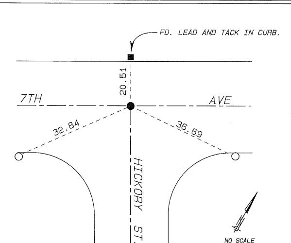
●-FOUND LARGE SPIKE IN PAVEMENT PER RECORD OF SURVEY NO. 18943. CORNER RECORD NO.34568 CALLS OUT 5/8" PIN. SPIKE DESTROYED BY STREET PAVING WORK, RESET SPIKE AND WASHER MARKED "CITY ESC" AT SAME LOCATION. SEE CORNER RECORD.
