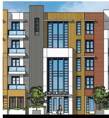
GLASS RAILS, ABV. ENTRY STOREFRONT & AWNINGS MTL SIDING
